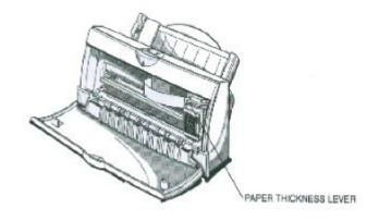
Set the lever according to the thickness of the paper you are using:
